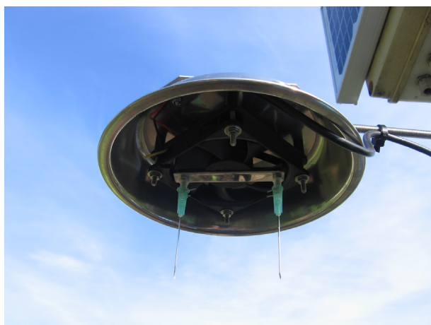
Figure 2. AMETRAP with injection needles coated with silicone grease
