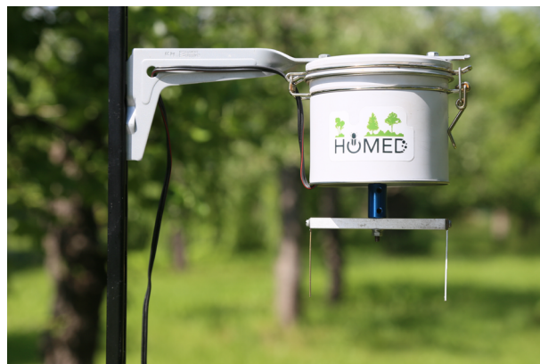
Figure 1. ROTTRAP 52 with square-profiled impaction rods coated with double-sided tape
